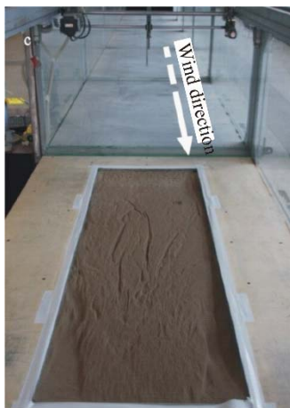
Fig. 1 Position of the bed in the wind tunnel
